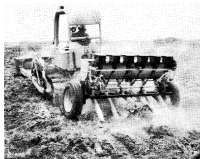
FIG. 11 Experimental rangeland seeder with semi-circular seedbox and auger agitator system plus flexing, runner openers for seed placement on log-littered surfaces. Unit operated without undue mechanical breakage on seedbed prepared by anchor chaining following root plowing of mesquite infested rangeland near Guthrie, Texas.
