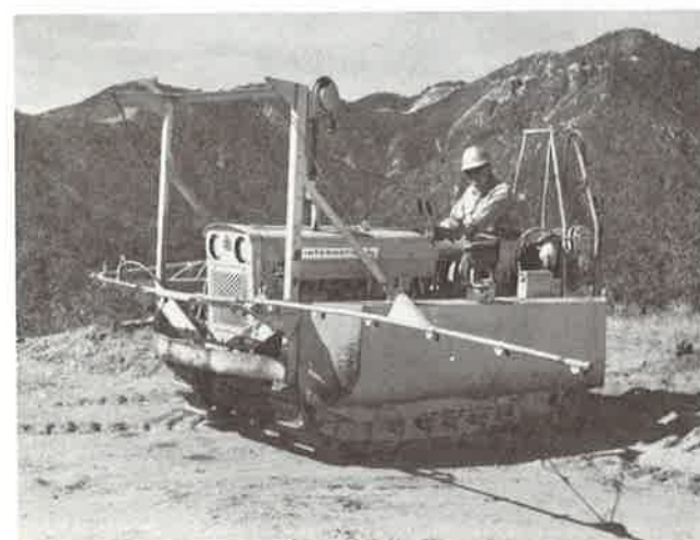
Improved sprayer system for a small crawler tractor.
