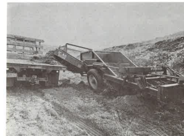
Sprigger harvesting sprigs to be planted on reclamation sites.
