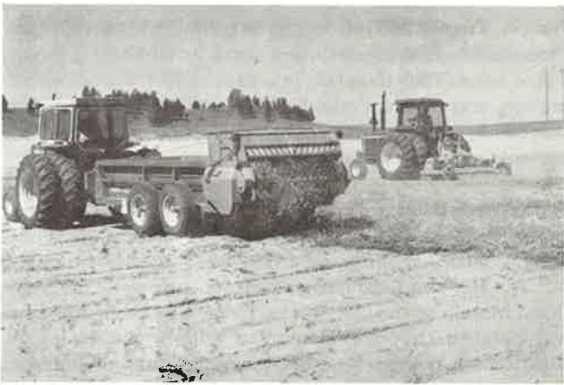
Modified manure spreader distributes straw mulch incorporated by a rotovator.
