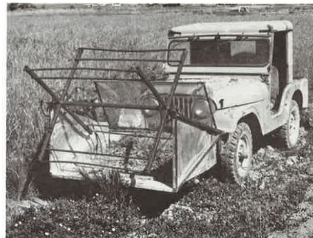
Reel type grass seed stripper mounted on a jeep.
