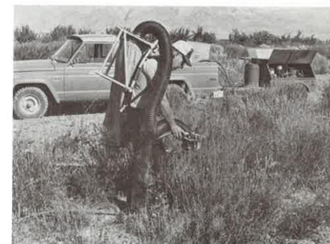
Seed collector connected to a large air compressor.
