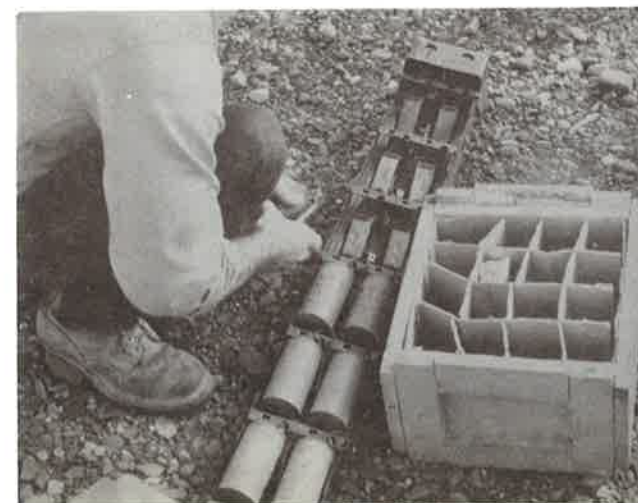
Placing thermite grenades in a dispenser.
