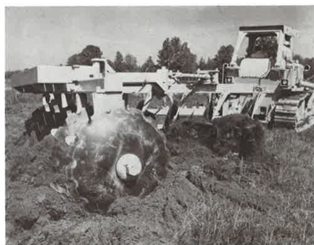
Cultivating action of large cut-out disks.
