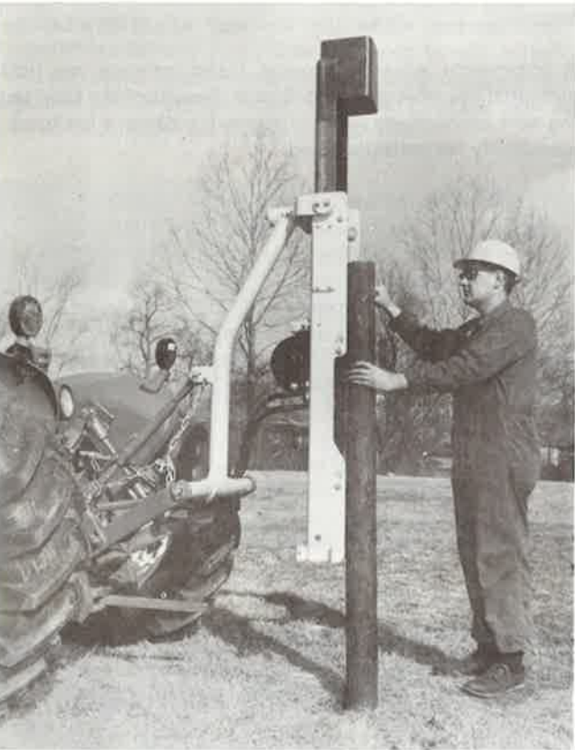
Post driver mounted on a three-point hitch.
