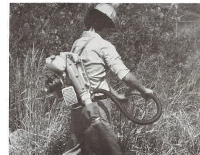
Solo backpack-mounted seed collector with 1-1/8-inch diameter inlet.
