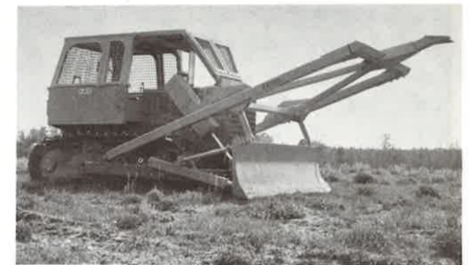
Push bar and dozer blade for clearing large trees.
