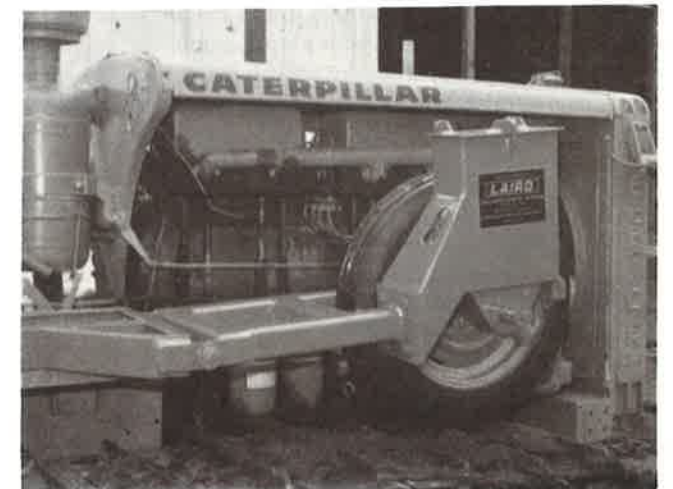
Seed dribbler mounted above a crawler-tractor track.
