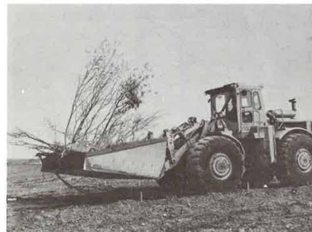
Dryland sodder placing stripped sod and vegetation on a reclamation site.
