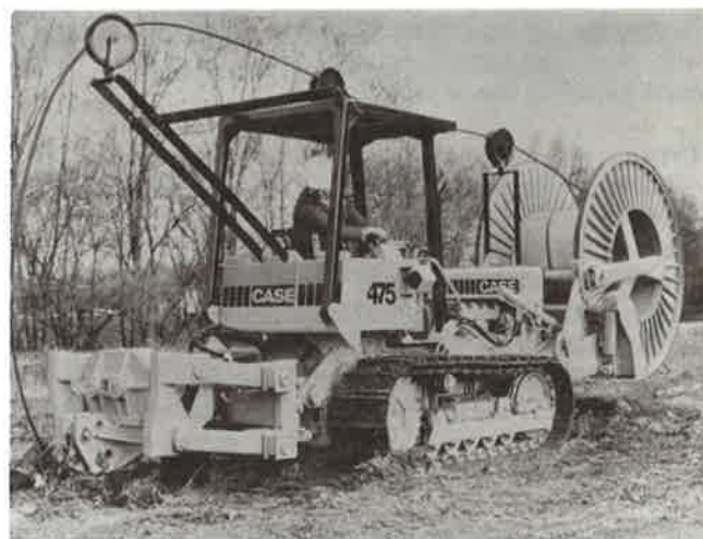
Cable plow may be adapted for laying plastic pipe.
