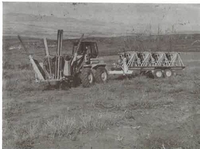
Towing the transport trailer with the front-end loader tree spade.
