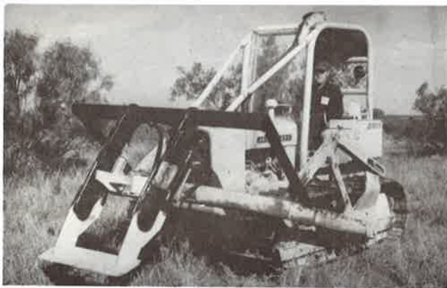
Low energy grubber for controlling mesquite.
