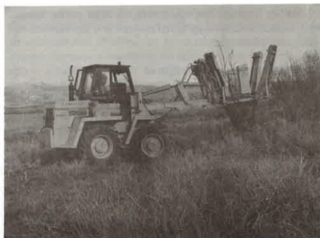
Tree spade mounted on a front-end loader.
