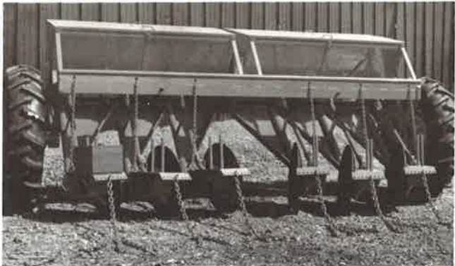
Rangeland drill with adjustable-angle deep-furrowing disk arms.
