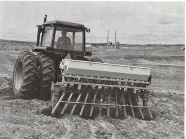
Modified gouger with automatic cycling mechanism and seedbox.
