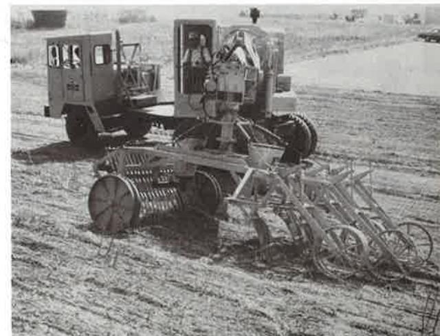
Steep slope seeder attached to a telescoping boom crane.
