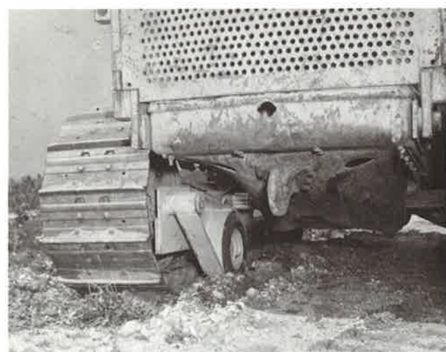
Precision grade indicator installed on a crawler tractor.
