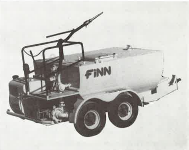
Hydro mulcher applies seed, wood fiber mulch, fertilizer, or soil amendments mixed in a slurry.
