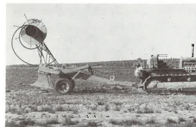
Towed ripper modified for laying plastic pipe.
