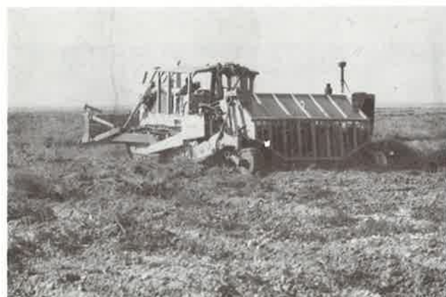
Stacko attachment for windrowing shrubs cut with a root plow.
