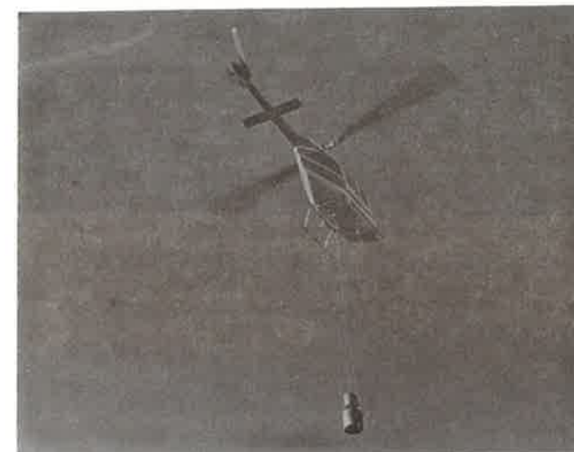
MEDC dispenser for ping pong balls loaded with \text{KMnO}_4 and injected with ethylene glycol.
