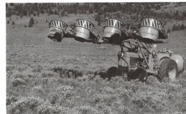
Four-blower thermal brush control unit kills brush without combustion.
