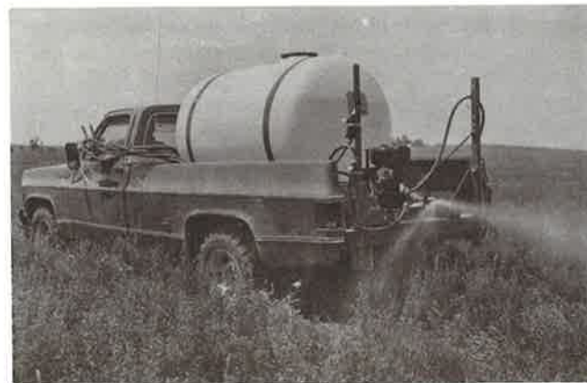
Skid-mounted sprayer with a wide-jet nozzle.
