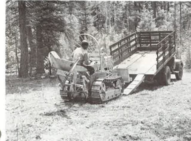
Tiltbed truck made from a modified stakeside truck.
