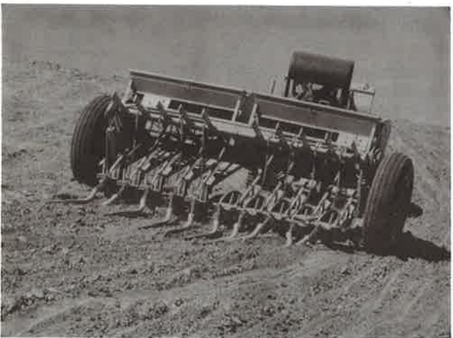
Fully equipped modern rangeland drill with deep furrowing attachments.
