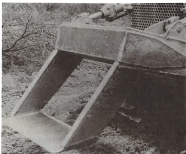
Grubber attached to a "C" frame.
