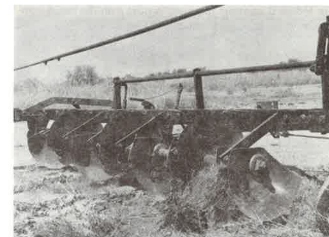
Cut-out disks for pitting the soil.
