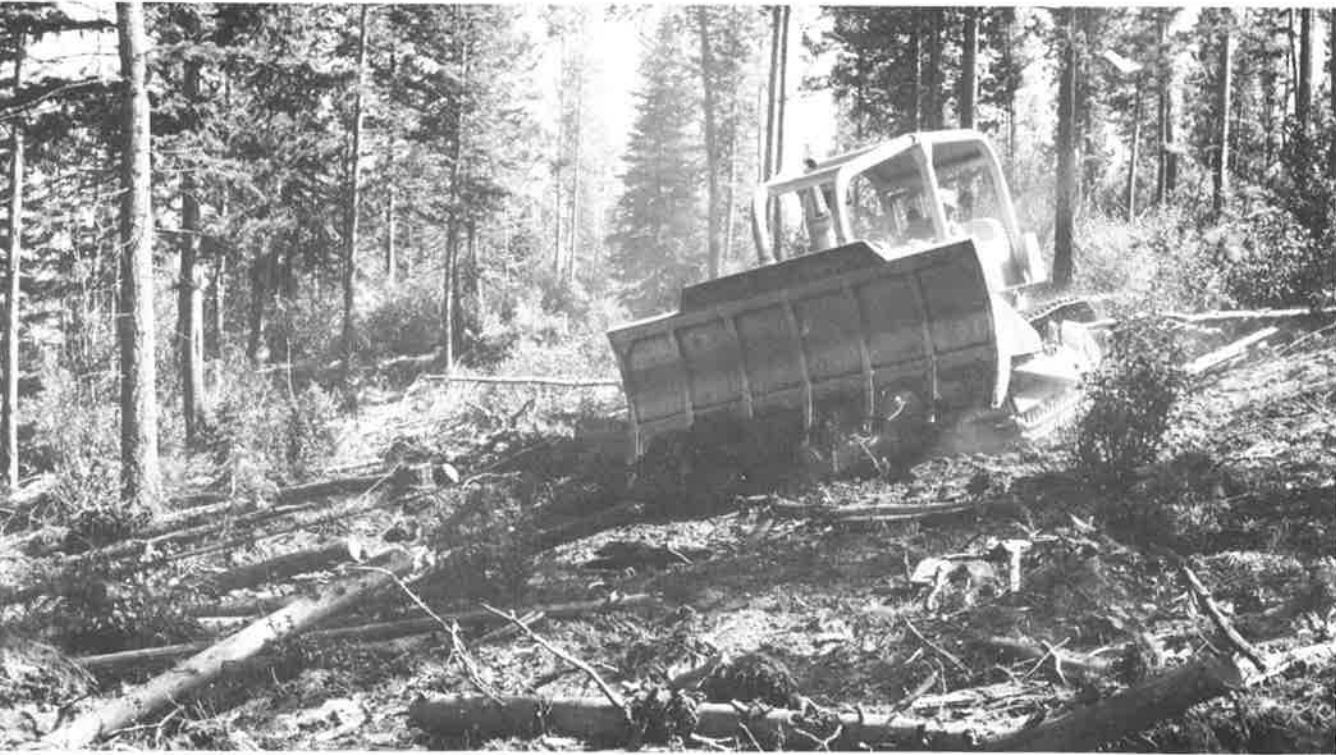
Blade design increases production with less disturbance to remaining trees.
