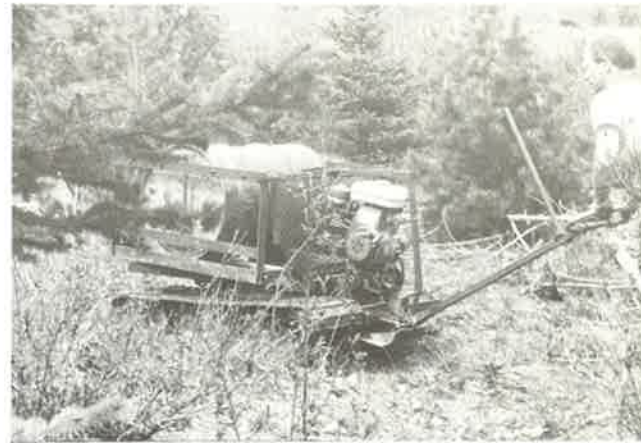
Portable power platform performs most forestry tasks.
