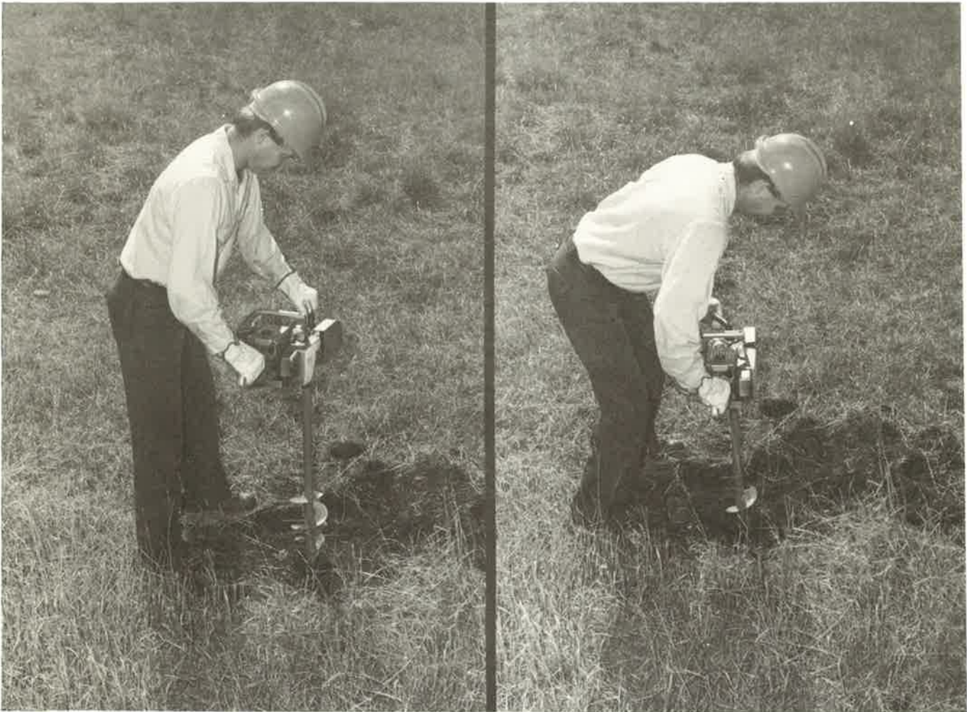
Cone-shaped, power-driven planting auger.
