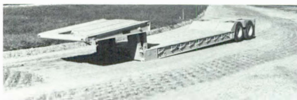
Lowbed semi-trailer with hydraulic gooseneck raised for transport.
