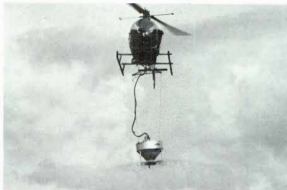
Rotary spreader suspended beneath a helicopter.
