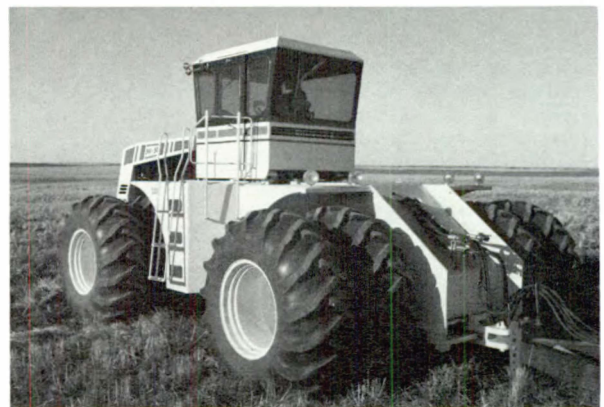
All-wheel drive tractor with articulated steering.
