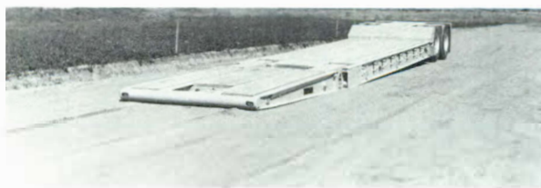
Lowbed semi-trailer with hydraulically controlled gooseneck in lowered position for loading.
