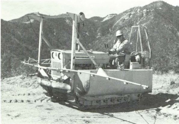
Side-mounted spray tanks on a small crawler tractor.
