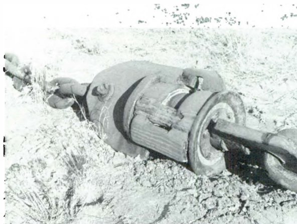
Chain swivel made from a large track roller.
