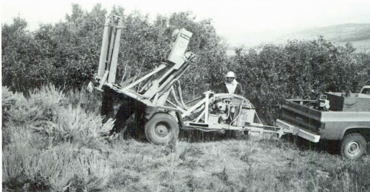
Trailer-mounted four-blade tree spade.
