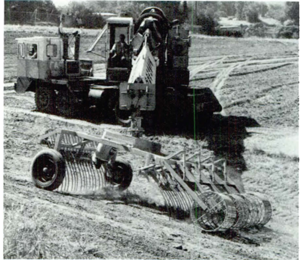
Steep slope scarifier-seeder.
