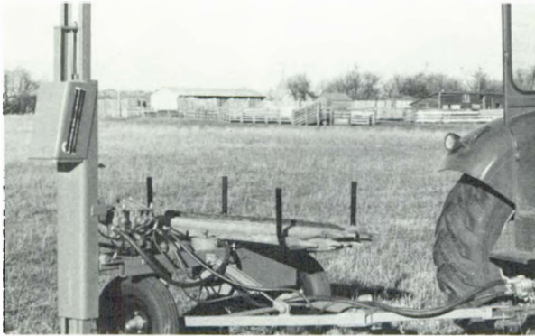
Post driver mounted on a separate trailer.
