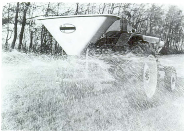
Oscillating pendulum spreader.
