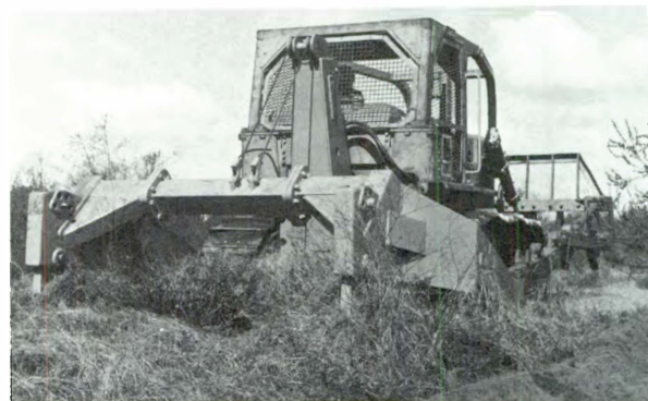
Root plow controlling brush by slicing roots.
