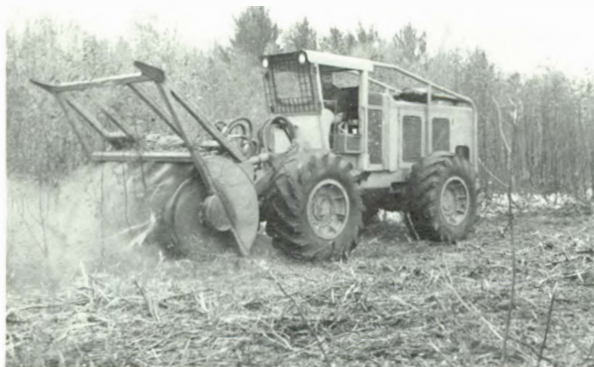
Self-propelled rotobeaer shredder masticating brush.
