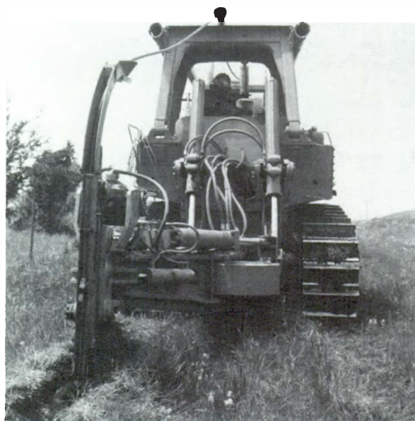
Cable plow with full hydraulic control.
