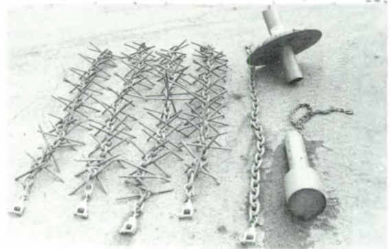
Klodbuster showing pick chains, lead chain, slope wheel, and weight.
