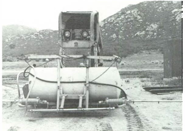
Single-point mountain spray booms attached to a crawler tractor.
