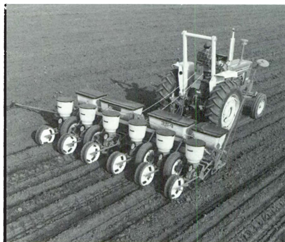
Air-powered planter units on a frame.
