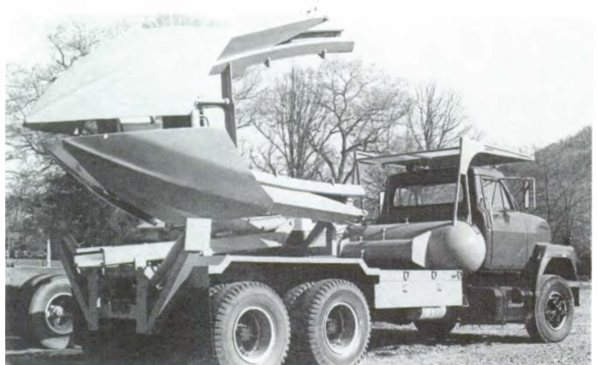
Large tree spade mounted on a truck.
