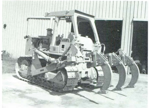
Subsoilers attached to a crawler tractor toolbar.
