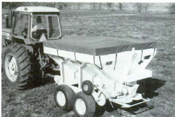
Trailer-mounted fertilizer spreader with a wheel-driven belt.
