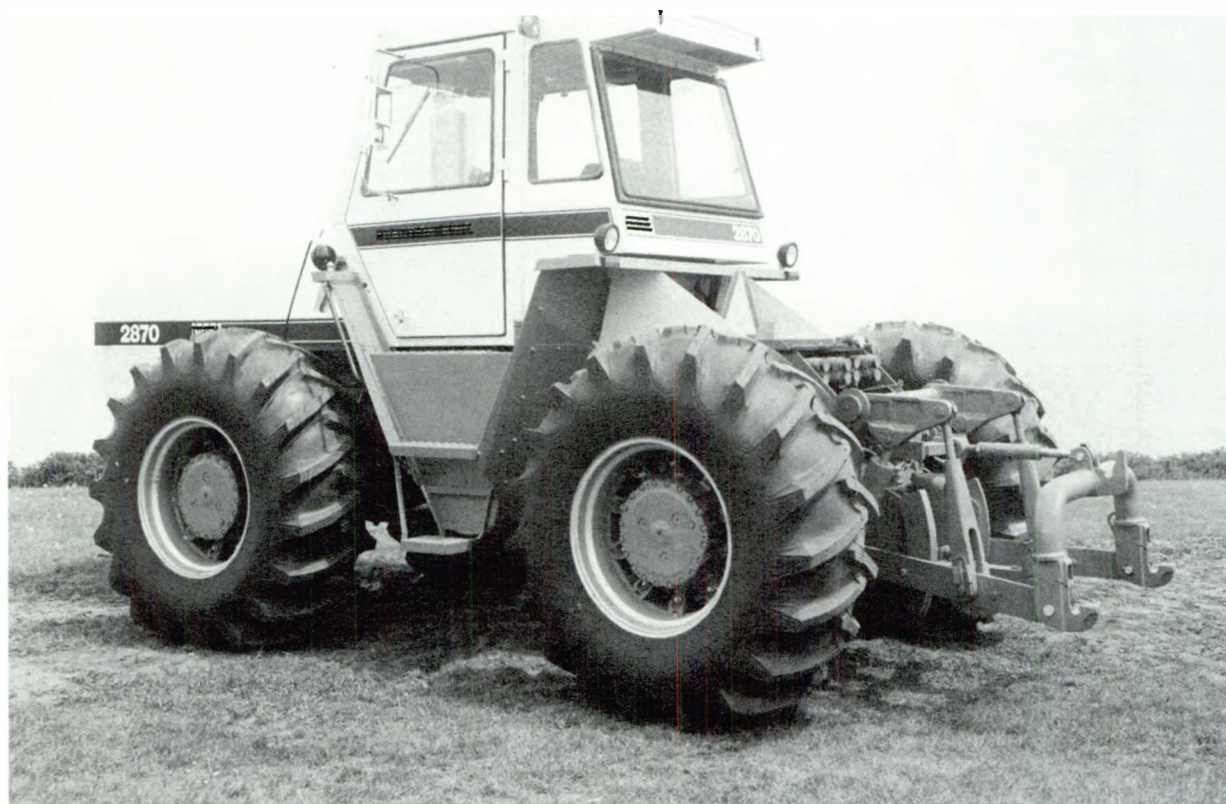
All-wheel drive tractor with independent steering of front and rear wheels.
