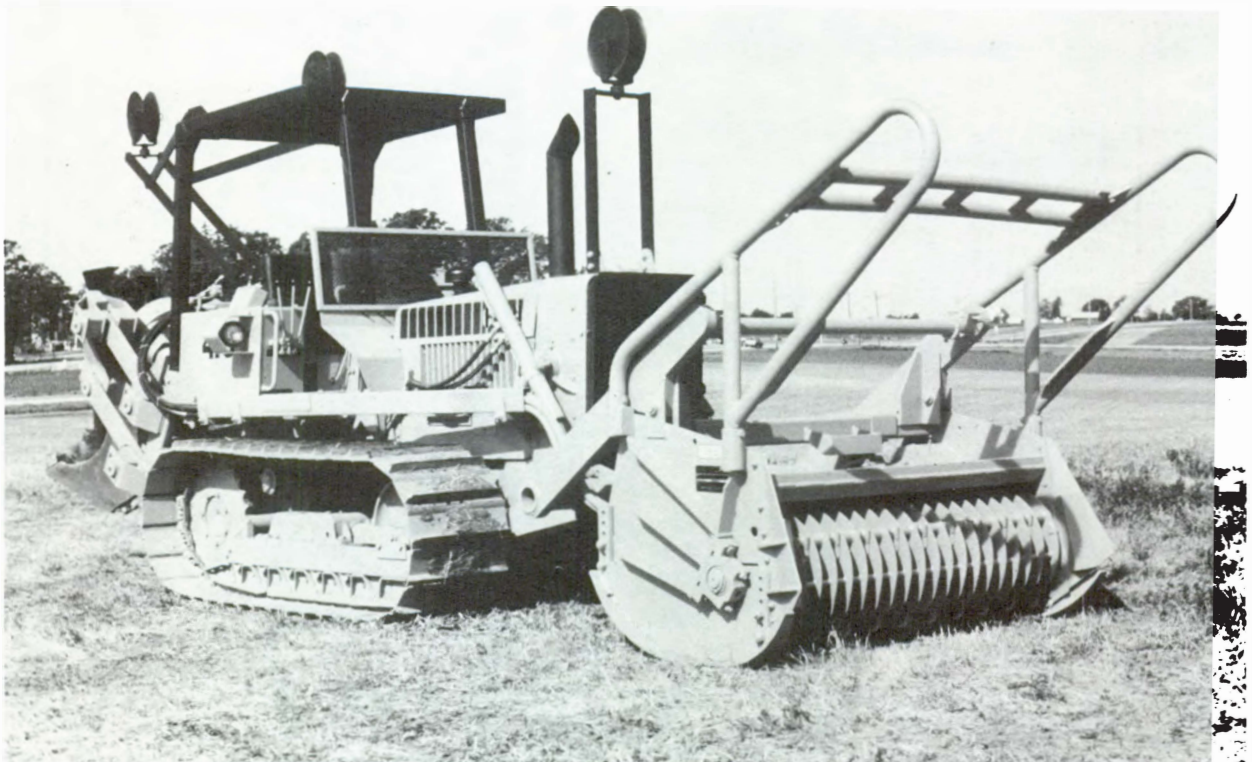
Rotobearer shredder mounted on a crawler-tractor.
