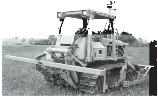
Three-point hitch for crawler tractors.
