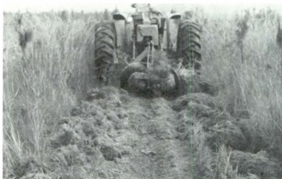
Fireplow cutting a wide, shallow furrow.
