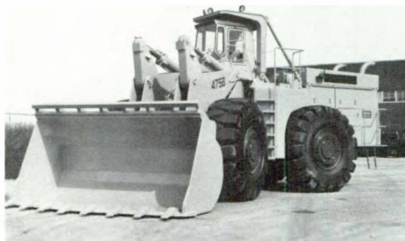
Large articulated front-end loader commonly available at mine sites.
