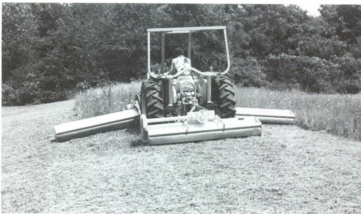
Three gangs of rotobeater mowers featuring both hydraulic and power-take-off drive.
