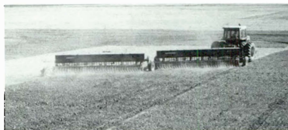
Seed and fertilizer applicators mounted on one-way disk harrows.
