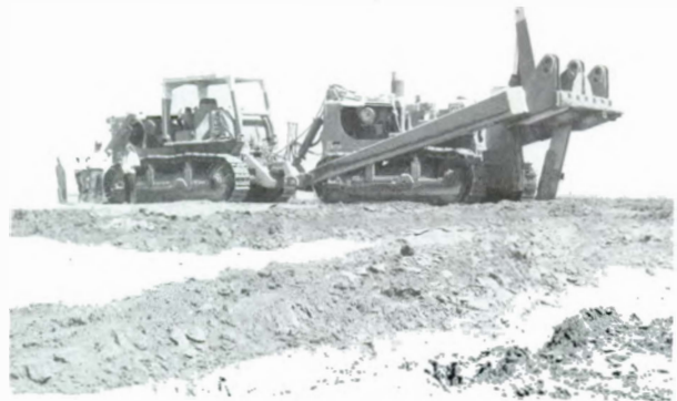
Large ripper for deep penetration.
