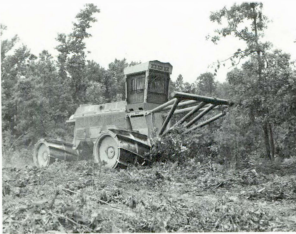
Large self-propelled rolling chopper.
