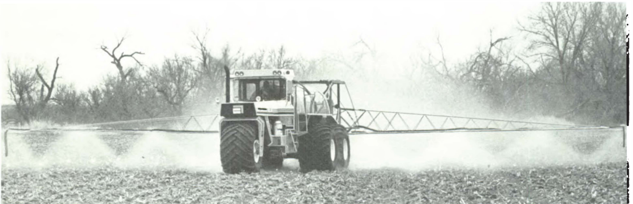
Large high flotation boom sprayer.
