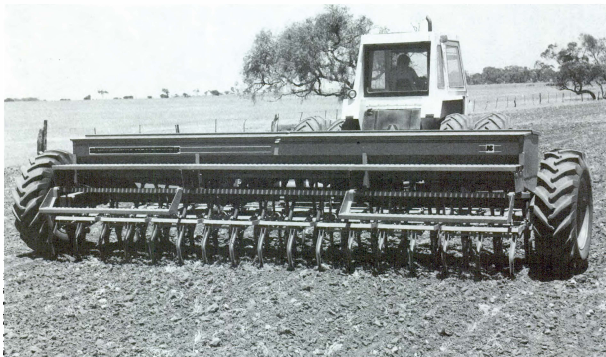
Grass drill with chisel openers.
