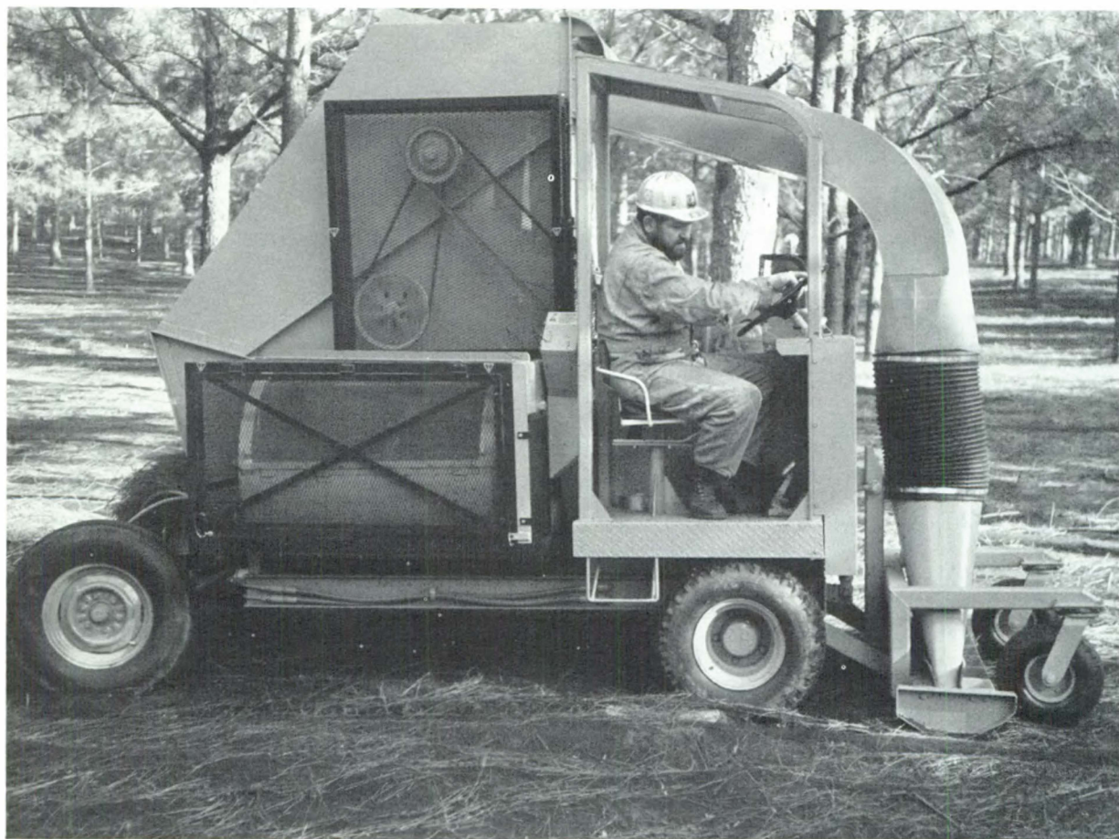
Self-powered vacuum seed harvester.
