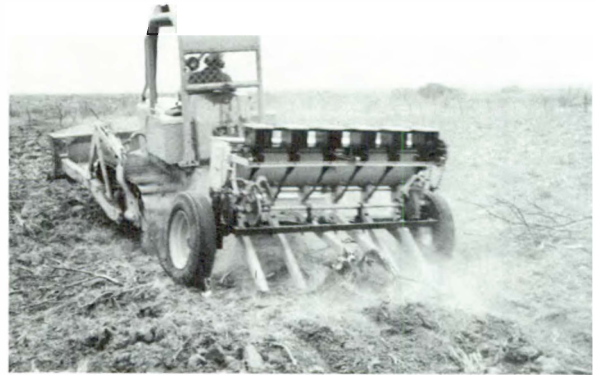
Range drill with flexible runners.
