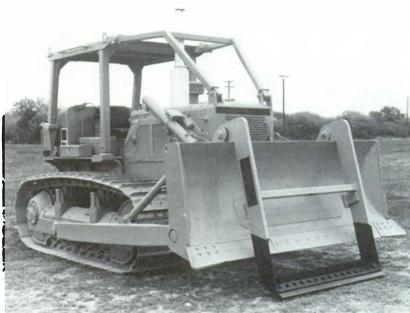
Detachable grubber mounted on a standard dozer blade.
