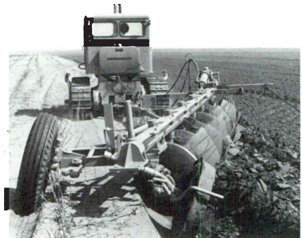
Large one-way disk plow with separate disks.
