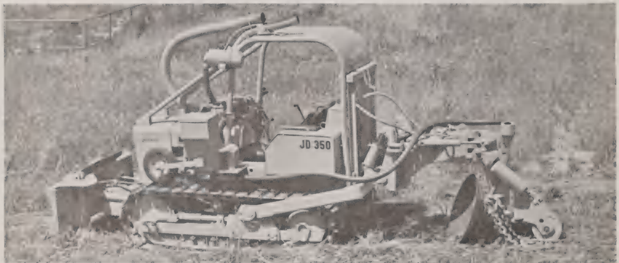
Interseeder prime mover is a John Deere model 350 crawler tractor.
