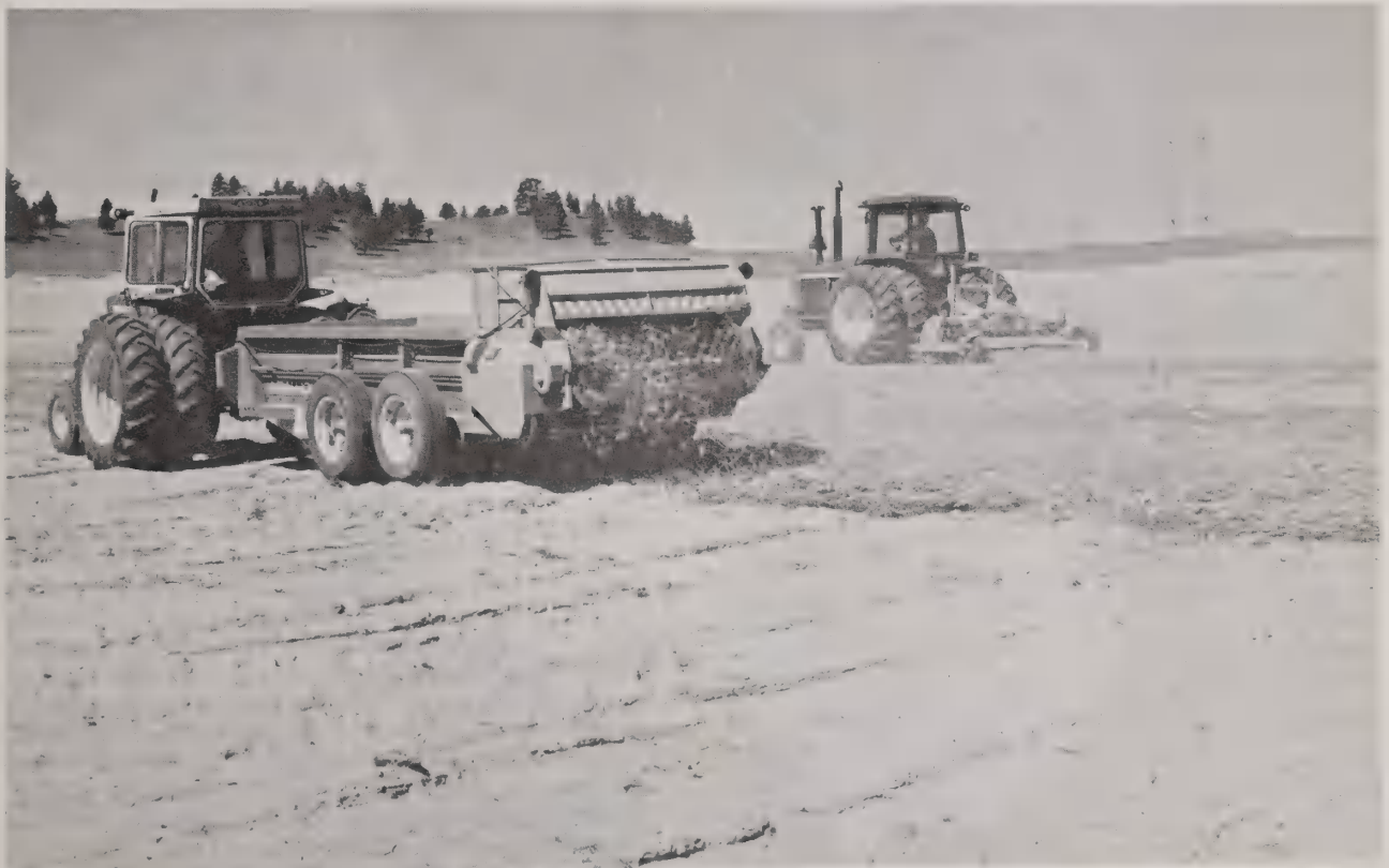
Rotavator (background) and mulch spreader combine to improve growing conditions on reclaimed mine site.
