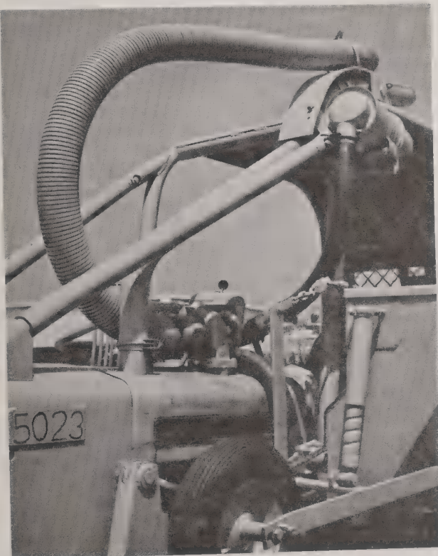
Turbocharger mounted on tractor with air filter and exhaust pipe.
