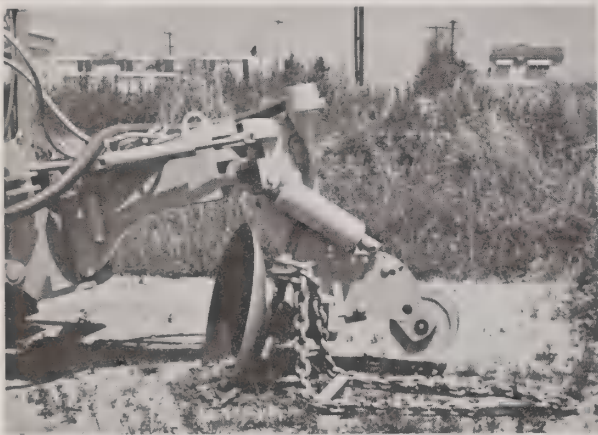
Gage wheel on single-disc trencher maintains constant furrow depth.
