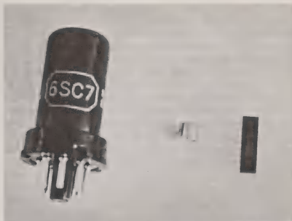
Automatic data recording systems were expensive, bulky, and unreliable when constructed with vacuum tubes (left) or transistors (center). Development of the integrated circuit (right) has enabled the construction of low cost, compact, energy-efficient, reliable systems.
