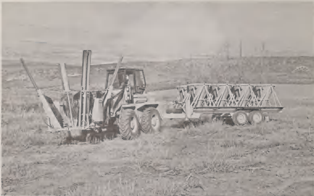
Equipment for transplanting trees and shrubs on reclaimed mine sites.
