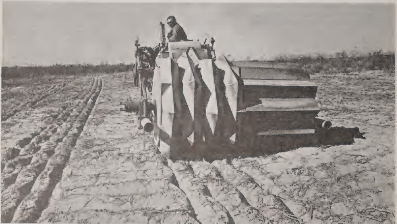
Land imprinter forming rainwater-irrigated seedbeds in an area infested with creosotebush near Tombstone, Ariz.
