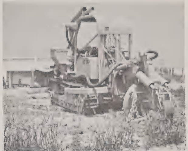
Plastic tubing carries seed from venturi tube to cyclone separator.
