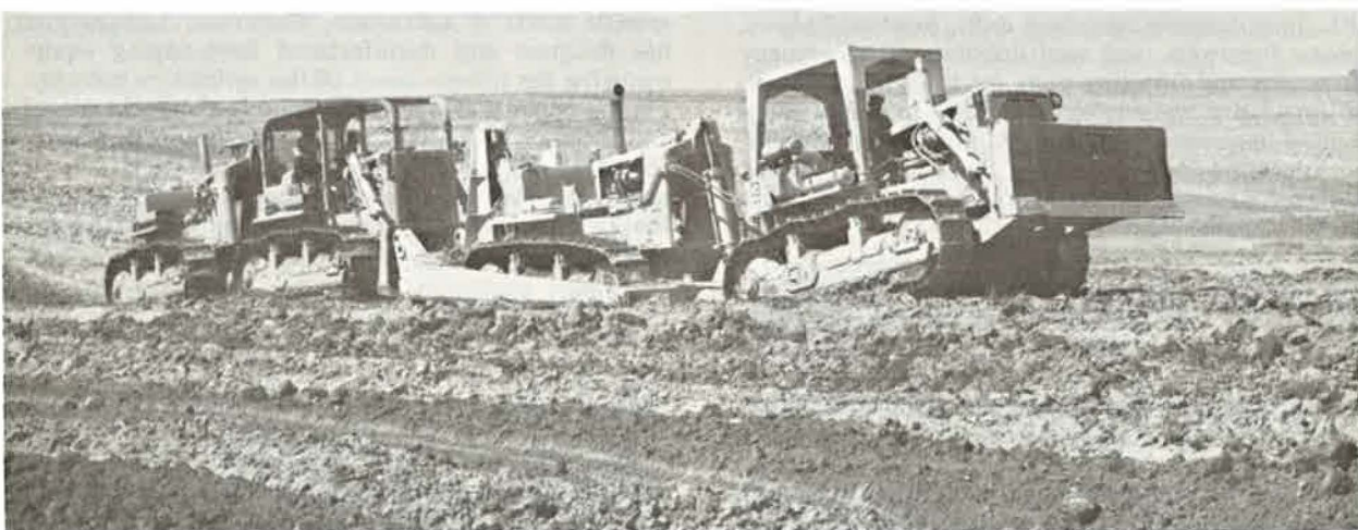
Tandem Caterpillar D-9's push Quadripper, giving 400,000-pound drawbar pull at 1 mph.
