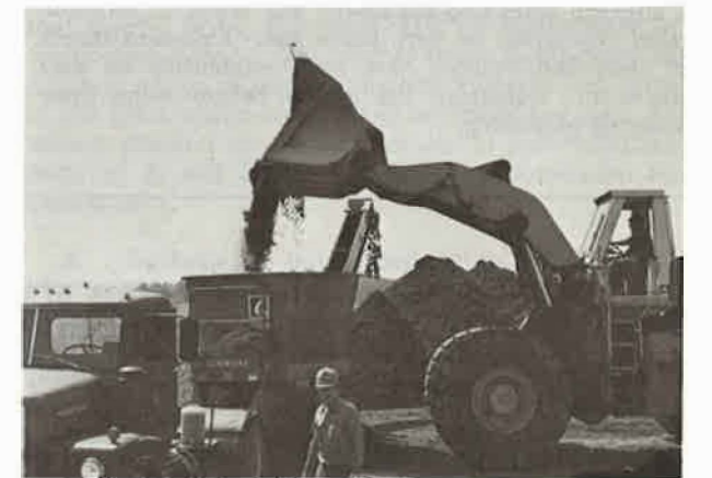
Bark is ground before mulching to eliminate large pieces of woody material that could damage spreading equipment.
