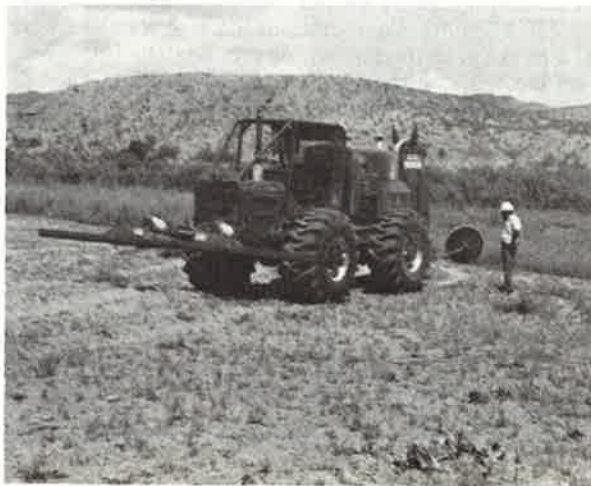
The 200-kilowatt, high voltage ac plant control unit mounted on a log skidder.
