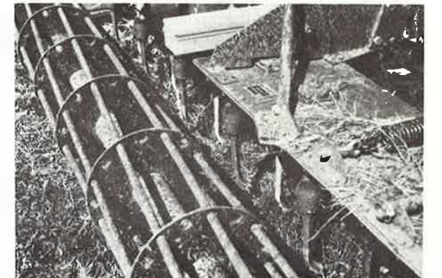
Figure 3.—Rear of vertical axis tiller. Mulching tines are in front of the roller.
