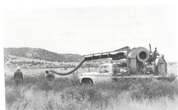
Jeep-mounted seed collector operating near Ephraim, Utah, September 1963.
