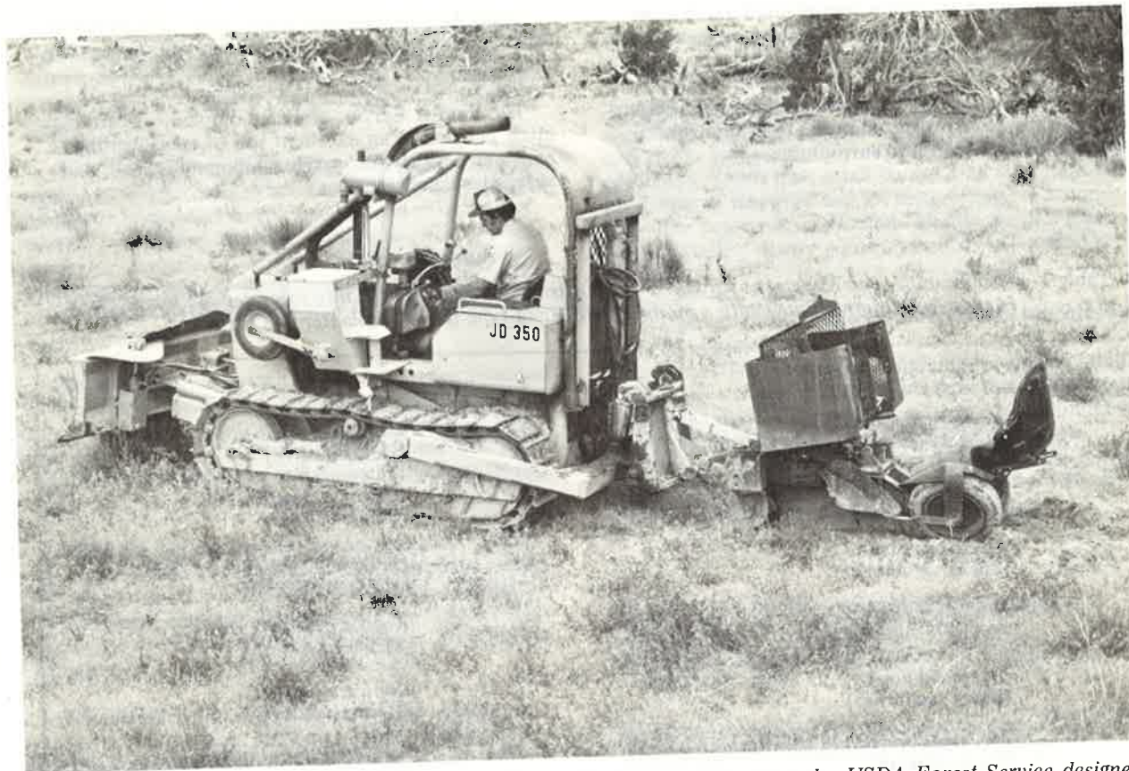
Transplanter used to plant shrubs in rangeland. It is attached to prime mover by USDA Forest Service-designed implement-carried hitch.
