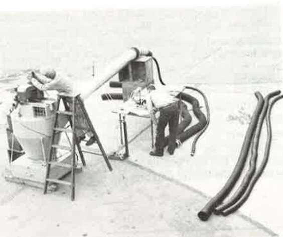
Jeep-mounted vacuum seed collector being tested at the San Dimas Equipment Development Center before field testing, June 1963.
