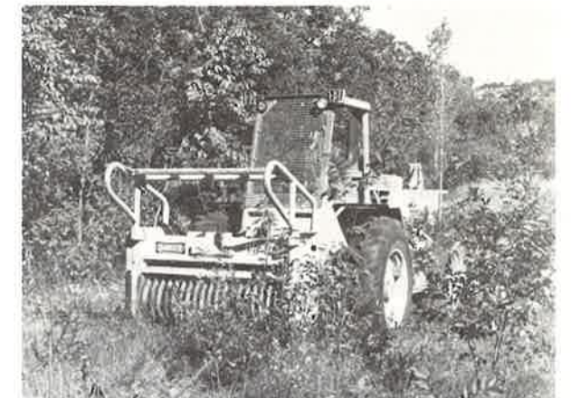
New combination of Brown Bear Cub four-wheel-drive tractor and Royer Woodsman shredder. Both are hydrostatically driven.
