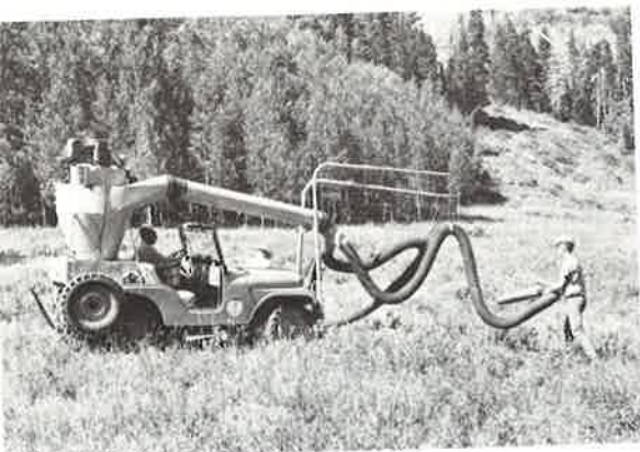
Jeep-mounted seed collector operating near Ephraim, Utah, September 1963.
