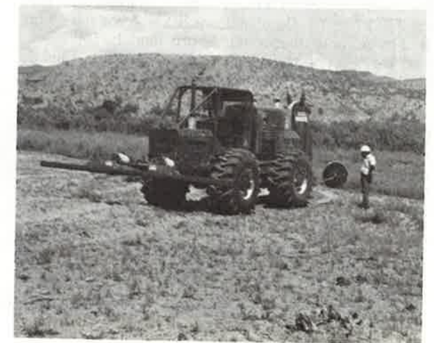
The 200-kilowatt, high voltage ac plant control unit mounted on a log skidder.
