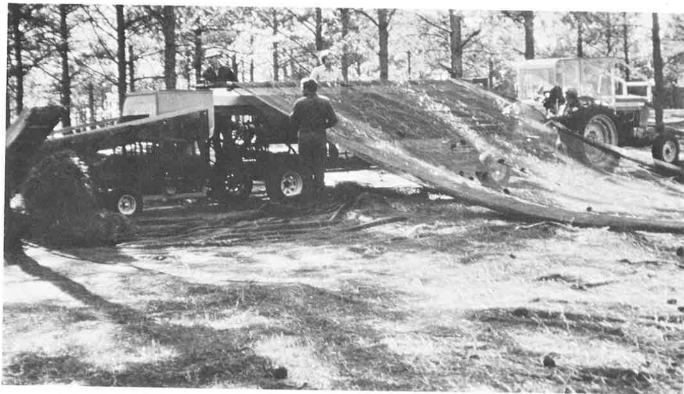
Seed collection system retrieves netting and separates seed from pine straw.
