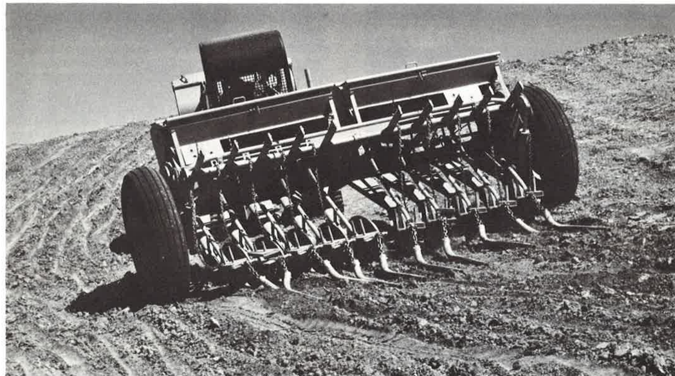
Rangeland drill is the most versatile seeding machine operated by D&C Reclamation.
