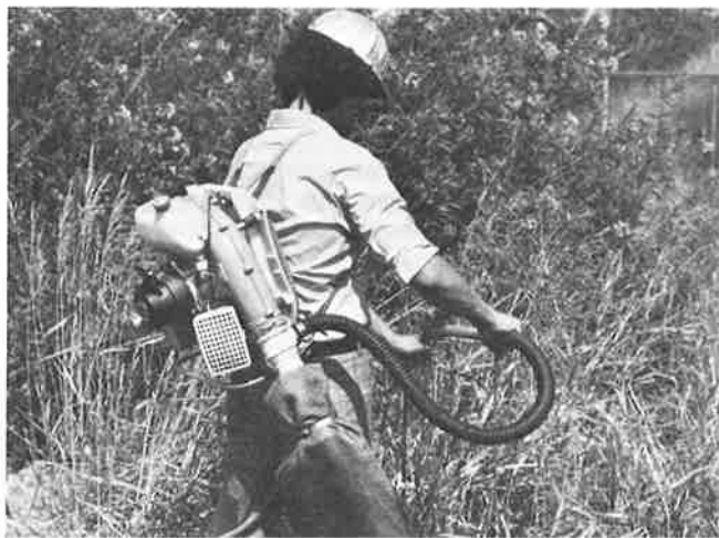
Figure 2.--Solo backpack-mounted seed collector with 1-1/8-inch inlet.
