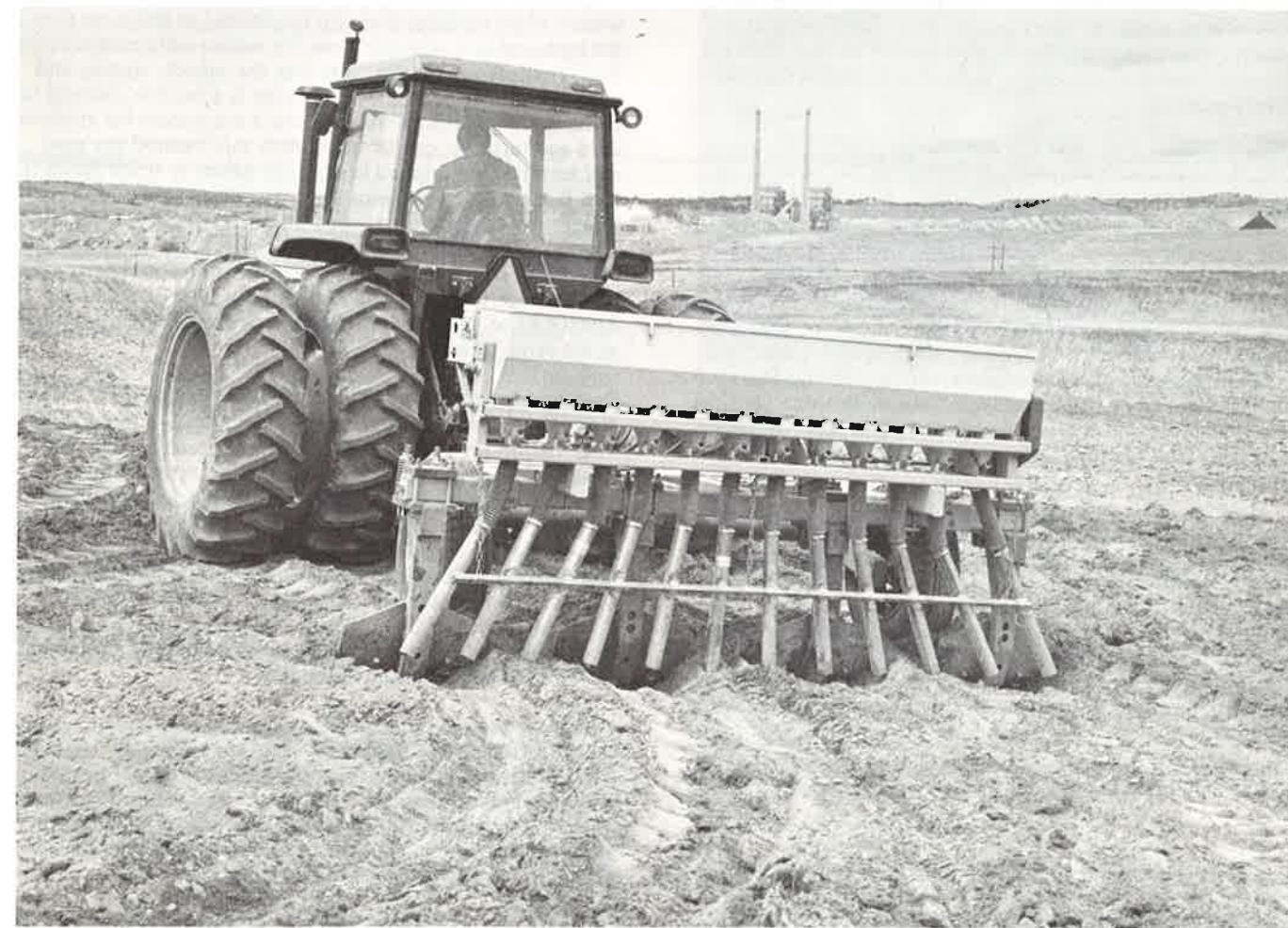
Hodder gouger makes depressions in soil and simultaneously seeds area to establish plant cover. Depressions create favorable microclimate that traps moisture and protects against wind.
