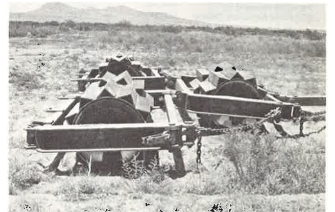
Converted rolling chopper imprints a 21-foot width.
