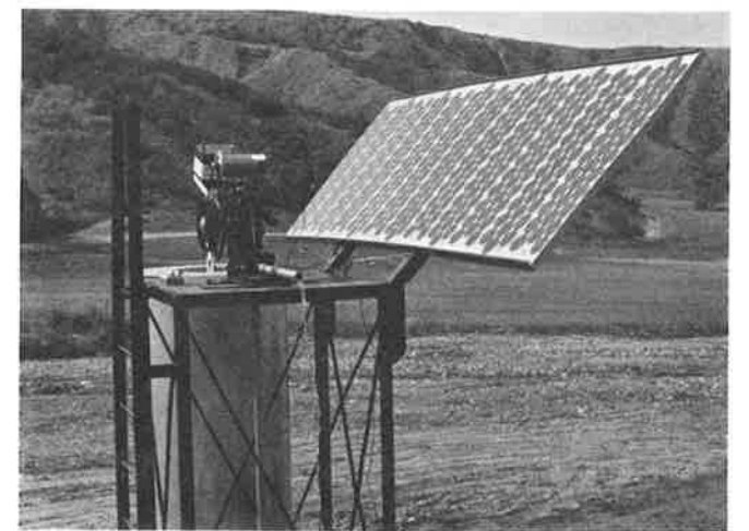
Photovoltaic solar powered conventional rod and well cylinder pump using no batteries and no controller. The unit pumps 2 to 3 gallons a minute from 230 feet, 5 to 7 hours a day, operating near Redlands, Calif.
