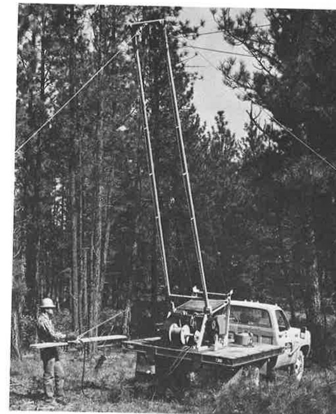
Mini Yarder is capable of pulling 2,000-pound loads at 160 feet per minute.
