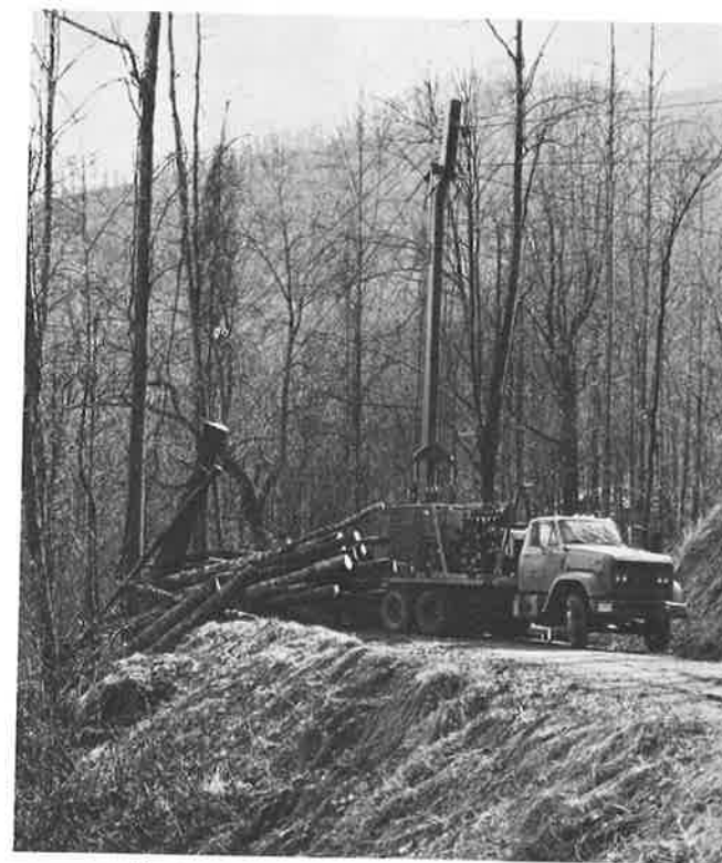
Clearwater Yarder can economically remove small logs and residue from steep rugged terrain.
