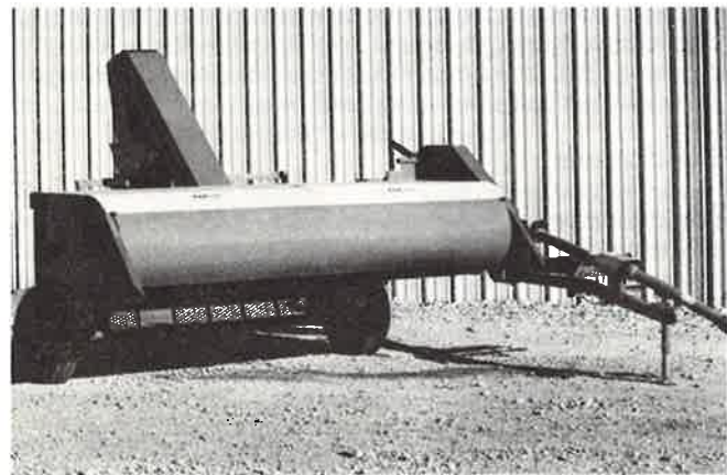
Kincaid grass harvester represents the application of seed harvesting research and development work by the Agricultural Engineering Department, Oklahoma State University. This harvester can be operated up to 4 ½ mph.
