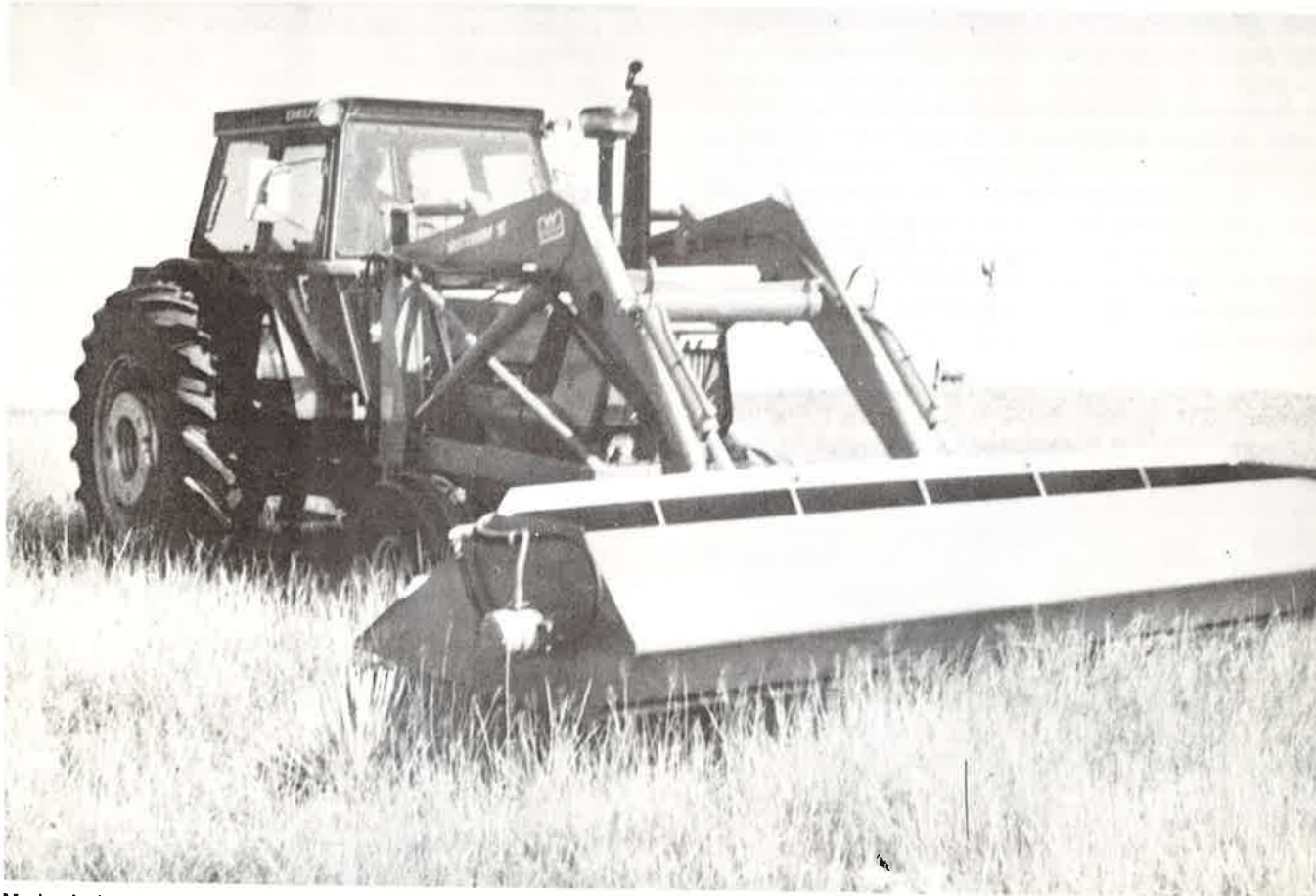
Mechanical seed stripper employing a rotating brush and airflow to collect chaffy seeded grasses in Woodward County, Okla.
