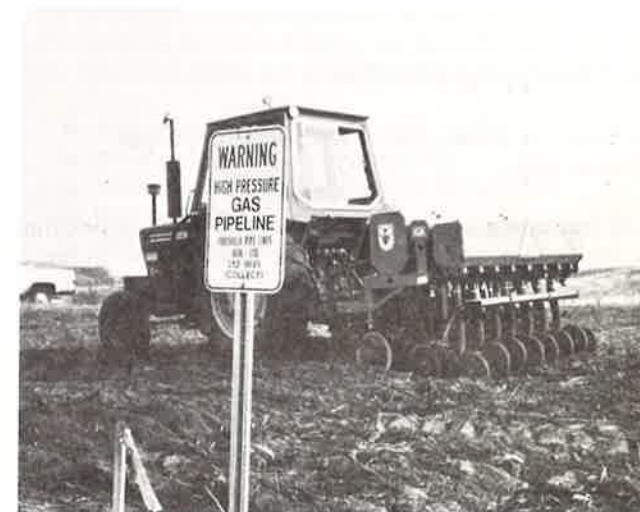
Tye drill seeding on the Alaskan Natural Gas Pipeline. This drill has three seedboxes to seed three different types of seed. The drill also dispenses fertilizer at the same time when equipped with optional fertilizer attachment (not shown).
