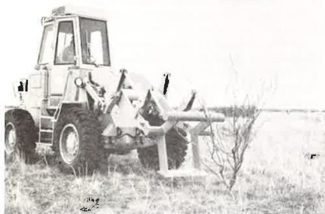
Rubber-tired loader grubber under study by Texas Agricultural Experiment Station appears practical for controlling small trees, such as mesquite, on rangeland that has been root-plowed and is being reinvaded.
