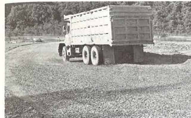
Lack of dust plume on woodchip segment of coal truck haul road.
