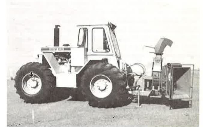
Brown Bear Cub tractor with Morbark Eger Beaver chipper mounted on front.
