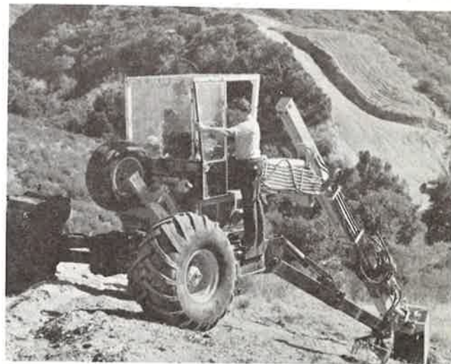
Mountain climbing backhoe that is able to climb steep mountain slopes like a five-legged spider and position itself to perform work.
