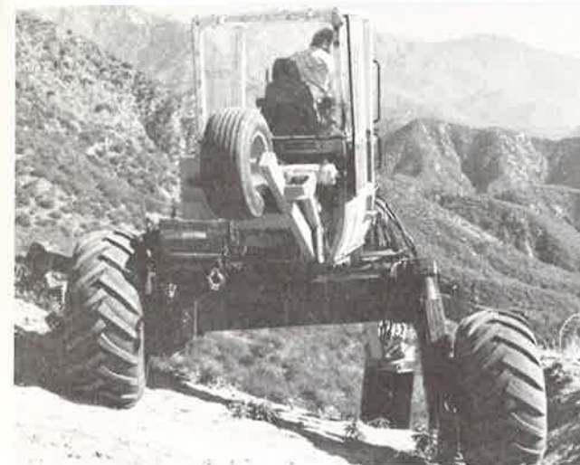
Each wheel or leg may be raised or lowered, extended or retracted, and/or moved in or spread out to accommodate radical changes in terrain.
