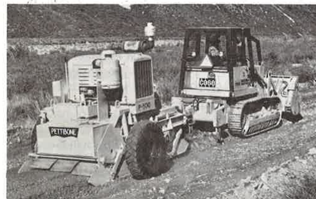
Mobile hammermill for treating oversized rock for use as road base.
