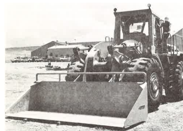
Figure 1.—Transplant attachment mounted on Terex 72-71A front-end loader.
