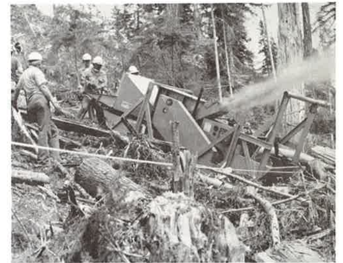
Onsite chipper for fire hazard reduction and residues reduction.
