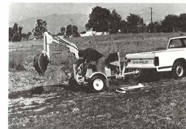
The Hopper Hoe can be towed behind a small pickup truck or car.
