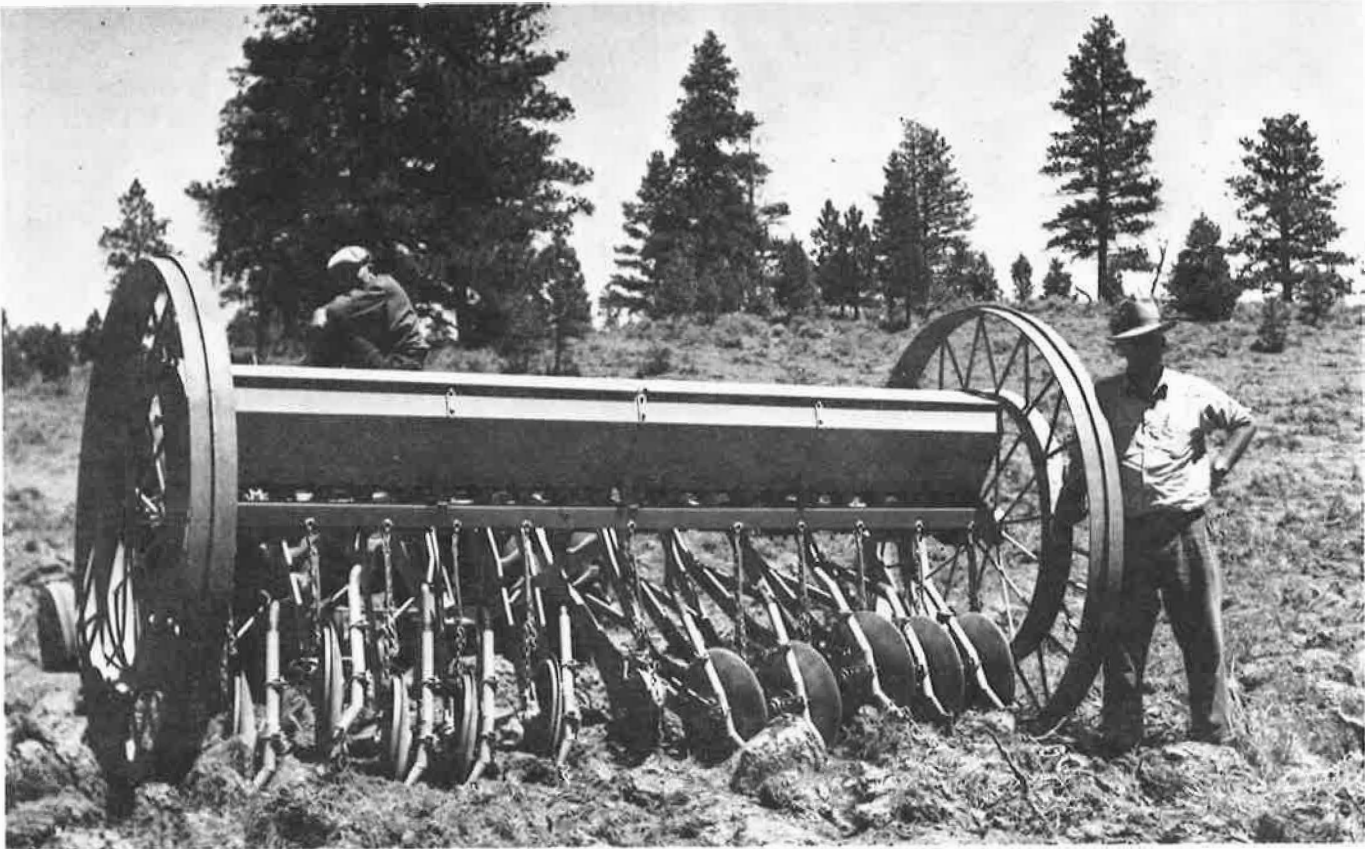
Demonstration model rangeland drill designed and built by John Kucera and N. R. Smith of the Fremont National Forest, Lakeview, Oreg., in operation on Coffee Pot Flat, 1951.
