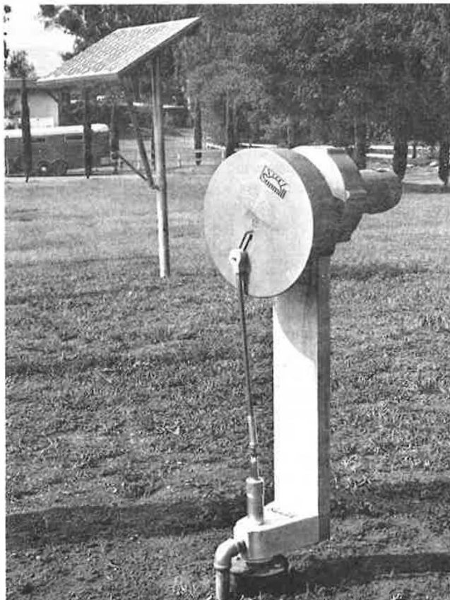
Production model of new type pump jack, powered by series-parallel photovoltaic panel switching.
