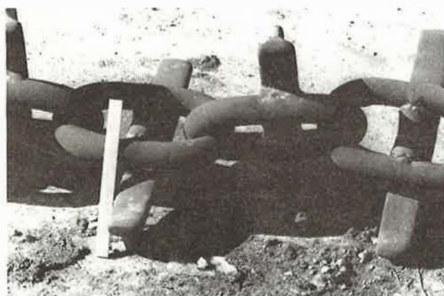
Many types and designs of digger teeth have been tried. The best "all around digger teeth are made using 18-inch-long railroad rails with the "foot" cut off and welded to the chain link. If the foot is not cut off, the chain will not "clean" itself of debris well. The chain links are 2½ inches in diameter and weigh 60 pounds per foot.
