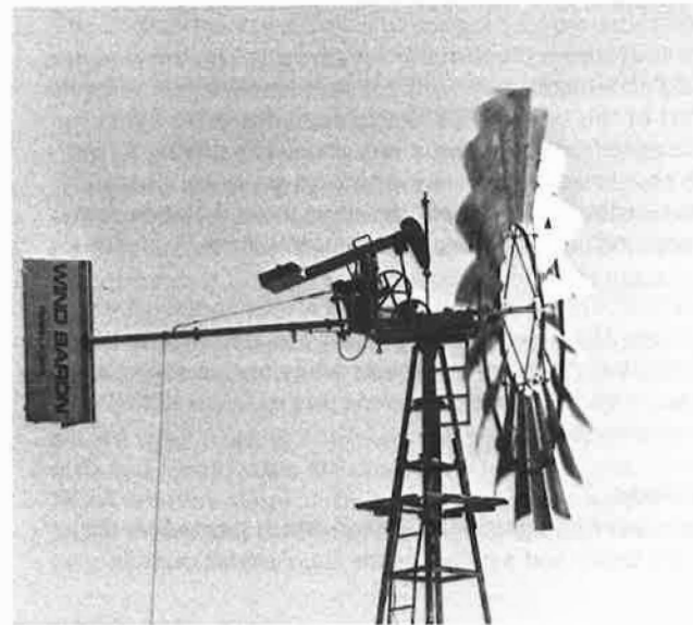
Wind Baron Mark IV Wind Machine. The walking beam counterbalance and aerodynamic tail are major factors in the Mark IV's ability to operate at low windspeeds. In periods without wind, an internal combustion engine, solar, or other power source can operate the Mark IV. Included as standard equipment is a separate power takeoff shaft, which can drive an electrical generator or other equipment.
