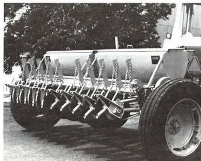
Hydraulically operated opener arms lift attachment for rangeland drill.
