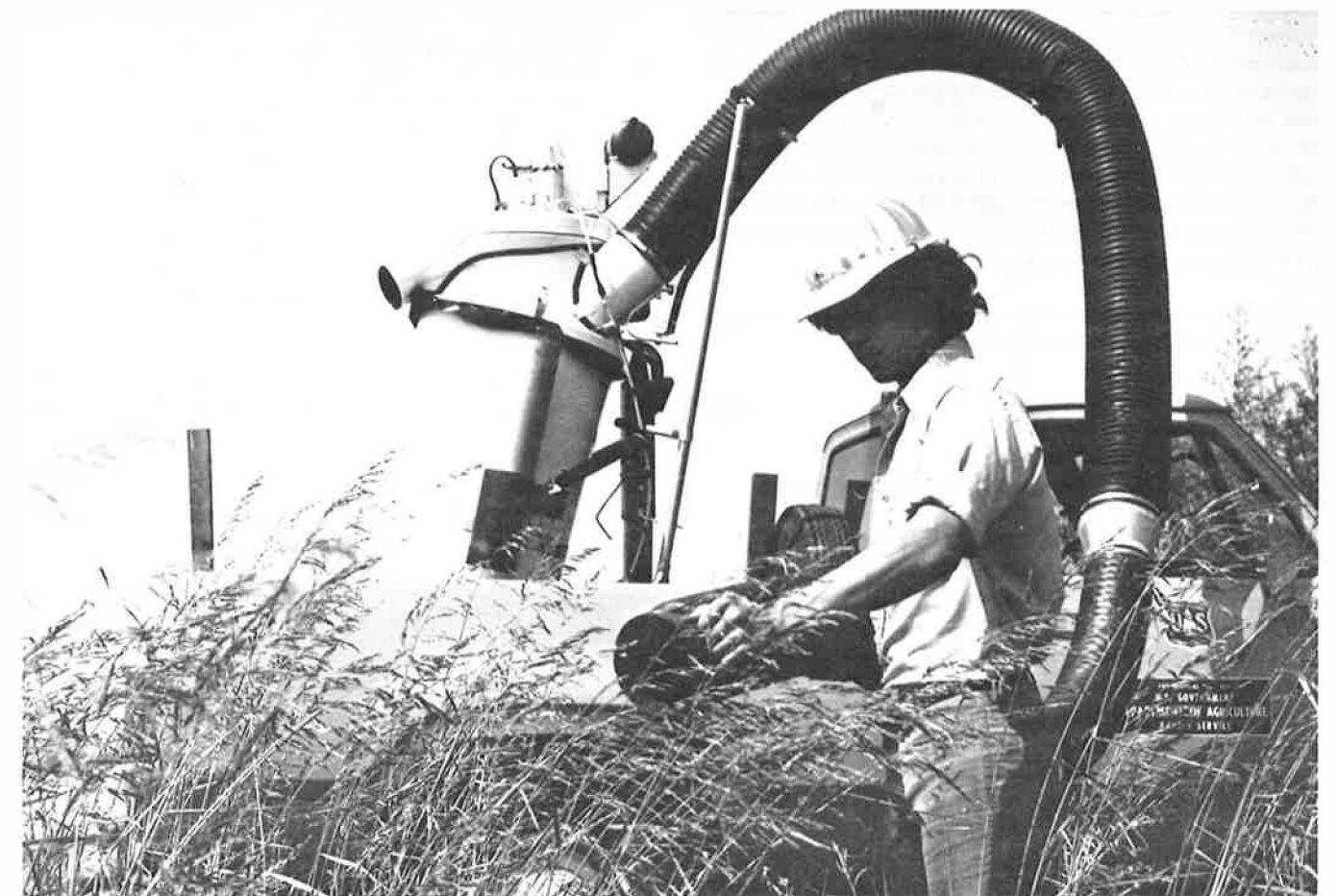
Elephant-Vac seed collector in operation.
