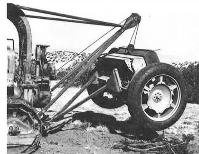
Half-size rangeland drill being carried so the tractor can back up. When the tractor is going forward and the drill is on the ground, the tractor can push juniper and seed in one pass.
