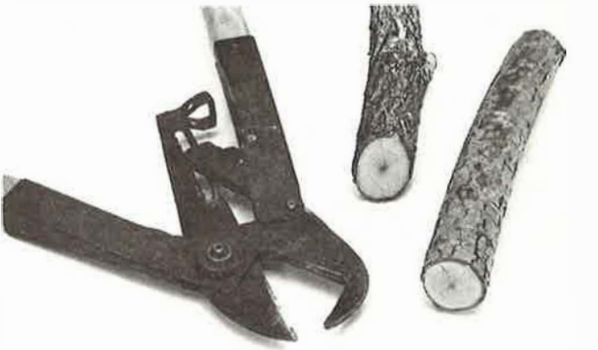
Hand-operated ratchet lopping shears will cut up to 2-inch stems using only moderate effort.
