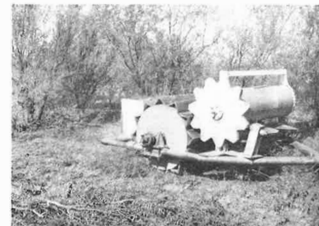
Brush-barrel seeder for disseminating trashy heterogeneous seed mixes.
