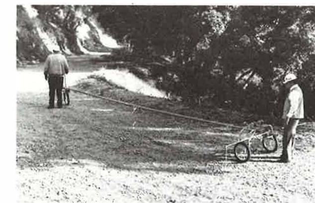
Design vehicle simulator determines if long-wheelbase vehicles can travel a road and make all turns.
