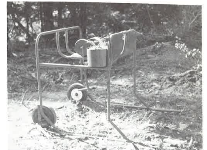
Burton Brush Bundler used to aid handcrews in treating slash.
