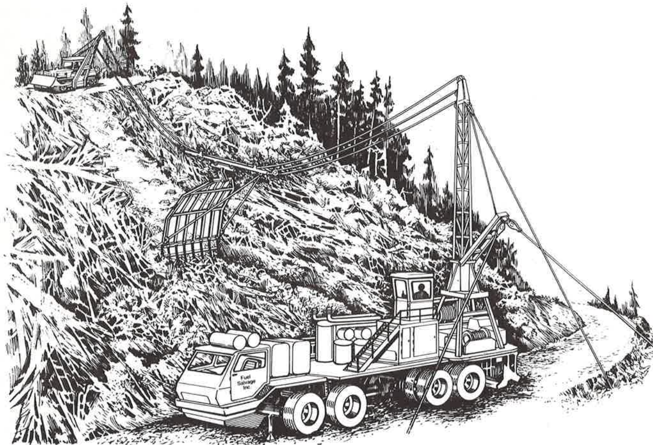
Artist's concept of operation of a slash rake attachment for a running skyline yarder.
