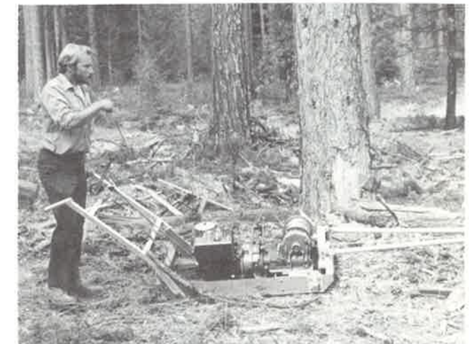
Slash concentrator in operation.
