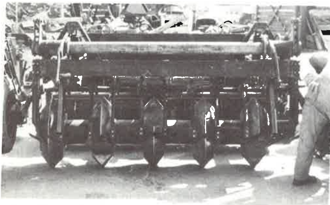
Figure 3.—Packing wheel unit configured for alternate row tillage with "cutouts" removed to form check dams on contour tilled native range.
