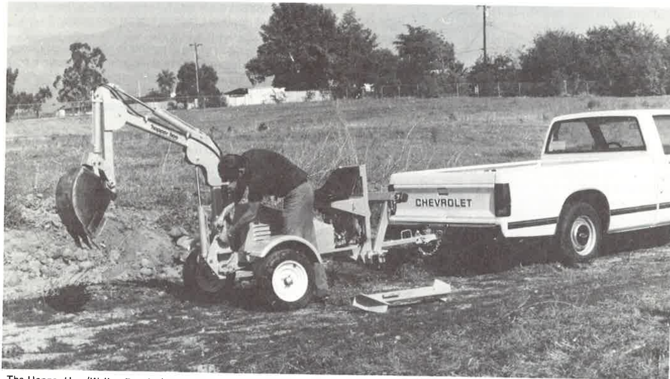
The Hopper Hoe (Walker-Dee Co.) can be towed behind a small pickup truck or car.
