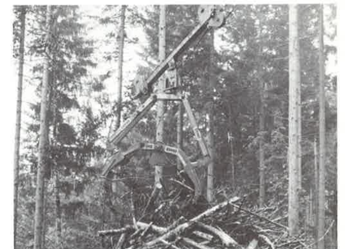
Slash grapple in operation on a running skyline yarder moving bundled slash to a landing.
