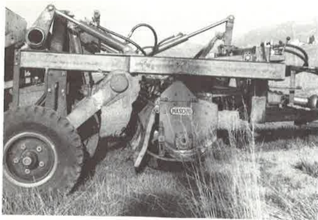
Figure 2.—Main frame showing hydraulics and lift configurations for tiller, transport wheels, and drill.
