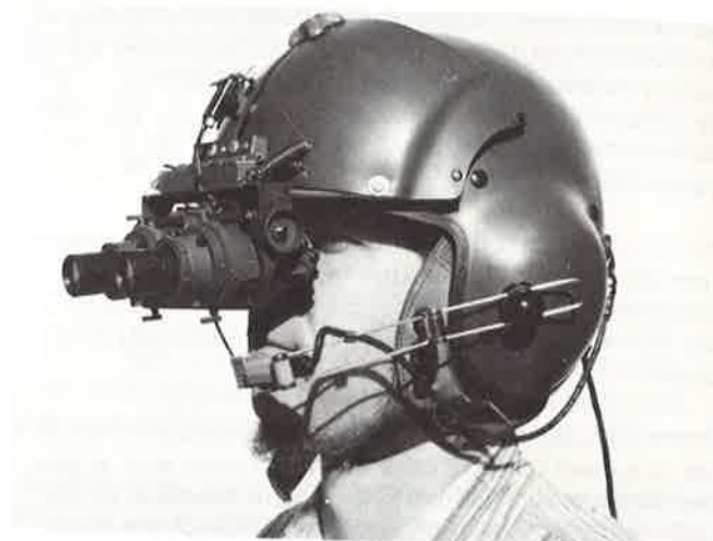
New lighter-weight night flying goggles in viewing position.
