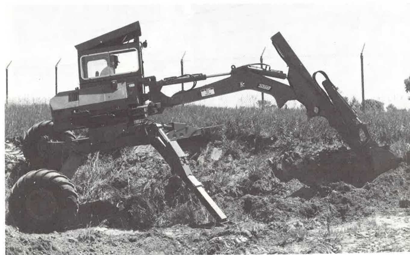
Schaeff-Namco walking excavator at work.
