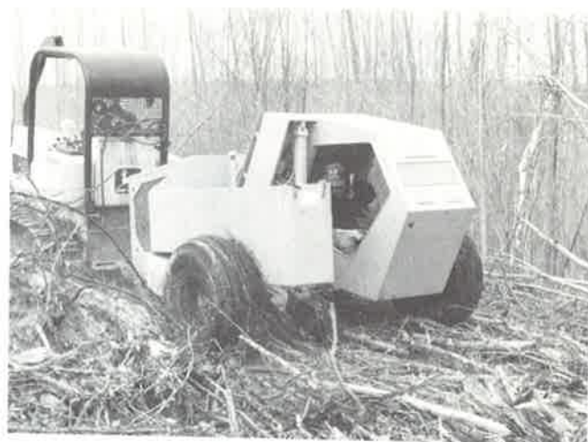
Marden Model 200 with onboard power supply intermittent-furrow tree-planting machine.
