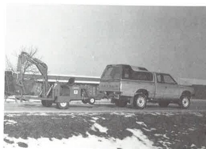
Mini-Hoe 600 can also be towed behind a small pickup or car.
