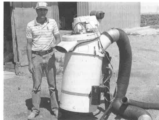
Figure 2.—The Elephant-Vac vacuum machine used in seed harvesting experiments on fourwing saltbush.
