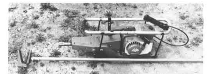
Figure 3.—Homelite shaker used in seed harvesting experiments on fourwing saltbush.
