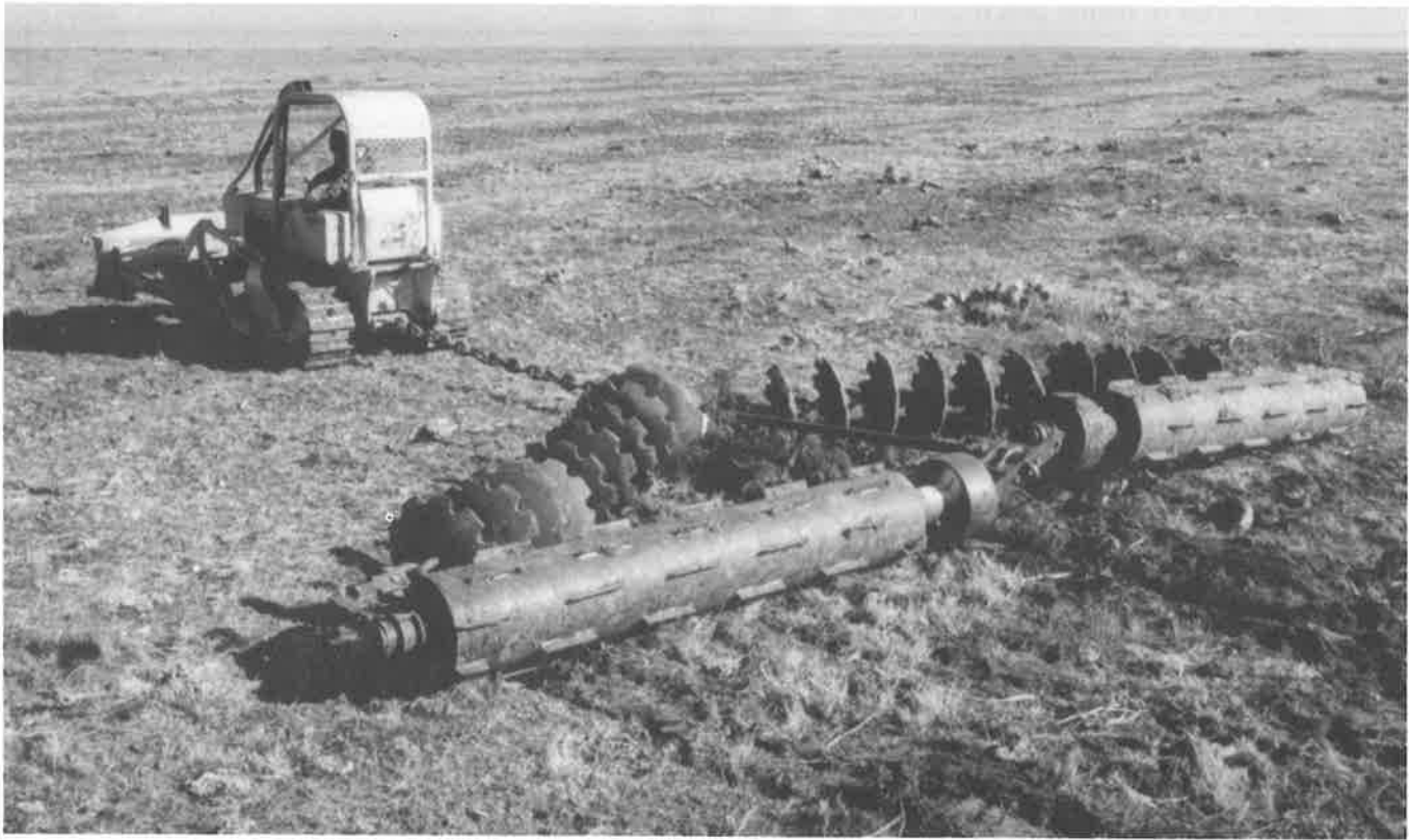
Disk-chain with flexing roller developed to prepare seedbeds on rangeland.
