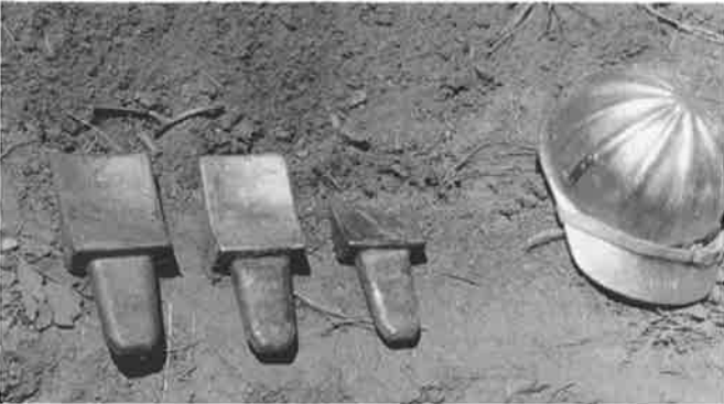
Teeth of Madge Rotoclear land breaking machine. These teeth can operate in material that can be cut with a hand ax.
