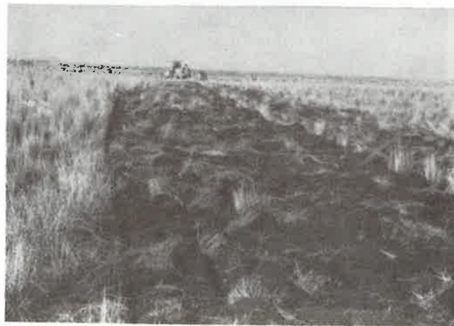
Disk chains are effective tools for preparing rangeland for seeding.
