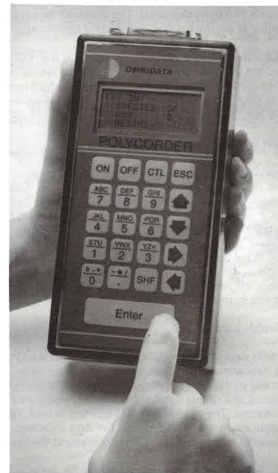
Omnidata International produces the polycorder, a portable data collector for laboratory and field application.
